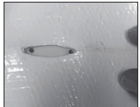
6. Push the tube together to hold the bottom repair plate in place and remove the screw.
