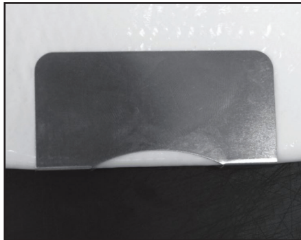
2. Place the template over the centre of the damaged area.
