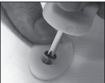
7. Place the top repair plate over so that the two guide holes line up. Replace the two screws then tighten with a screwdriver to complete the repair.
